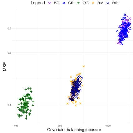
Figure 5: Scatter plot of MSEs over the covariate balance objective (nuclear norm) evaluated under different designs.
